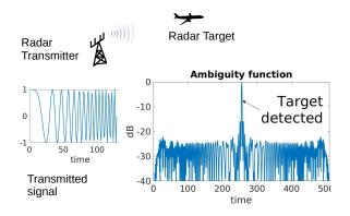
Waveform transmission  $\rightarrow$  Scattered signal recovery  $\rightarrow$  Matched filter response
